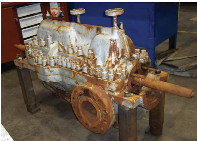
Pump as it arrived at the C&K repair facility from the refinery. Note the severely rusted shaft protruding from both sides.
