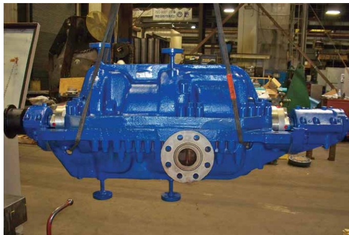
Repaired pump ready for shipment.
